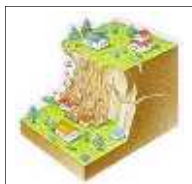
がけ崩れ Slope Failure
